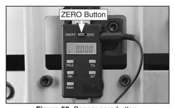
Figure 58. Sensor zero button.
